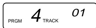
Select track number directly or with the SKIP button. Press PROGRAM to store
