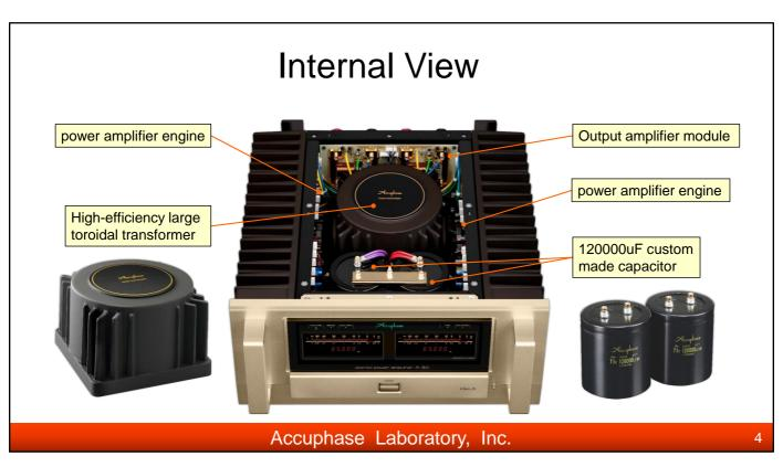
It has an intense power supply, a massive special-made high-efficiency toroidal transformer, and two sizeable 120000µF special-made filtering capacitors in the unit's center.
