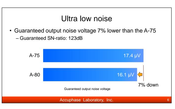
The former model A-75 has excellent noise performance; however, the A-80 achieves even 7% lower guaranteed output noise voltage than the former model.
