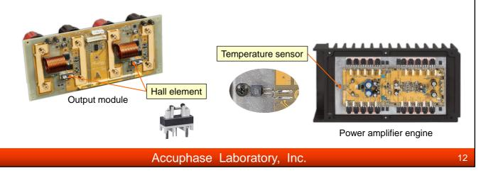
The Hall element on the output module detects overcurrent in the event of an output short circuit, minimizing any adverse effects on the music signal.
