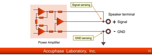
Remote sensing is the technique to lower the amplifier's output impedance by the negative feedback with the signal sensing from nearby the speaker terminals.
