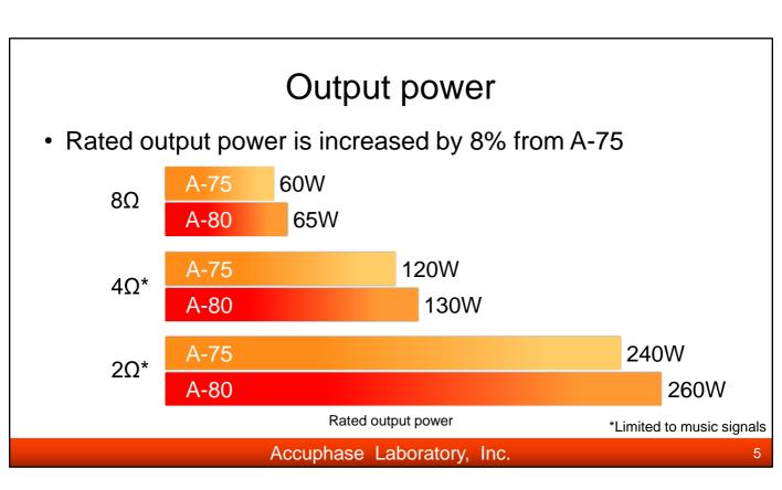
The A-80 improves the Class-A operation area by 8% over the A-75 as 65W into  $8\Omega$  load.
