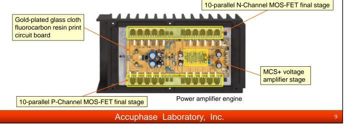
The 10-parallel push-pull arrangement of MOS-FETs in the power amplifier engine's final stage reduces the output impedance, thereby increasing the damping factor.
