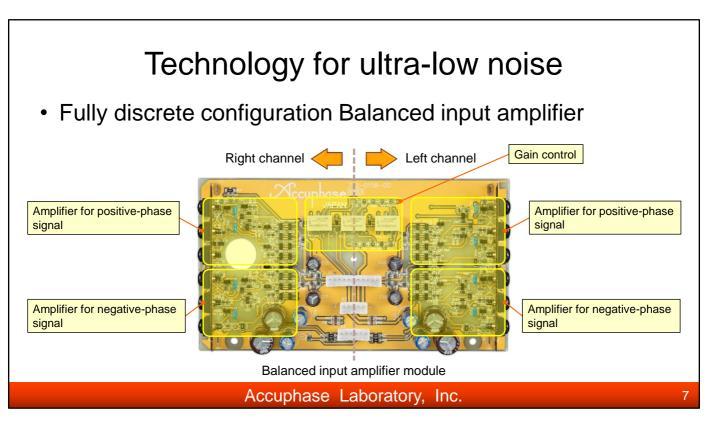
The output noise is reduced by a balanced input amplifier of fully discrete construction, newly designed in the A-300's circuit configuration.
