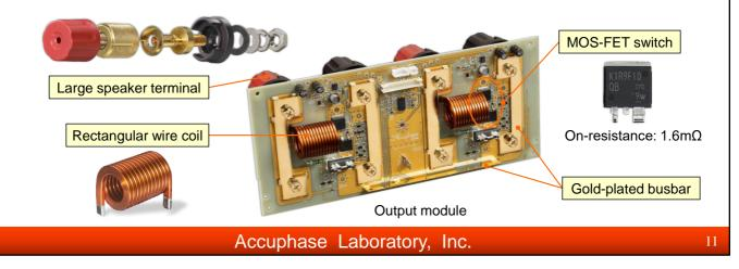
A mechanical relay is a typical speaker protection component, but its contact resistance is higher than people think.
