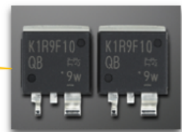
MOS-FET switch On-resistance: 1.6mΩ
